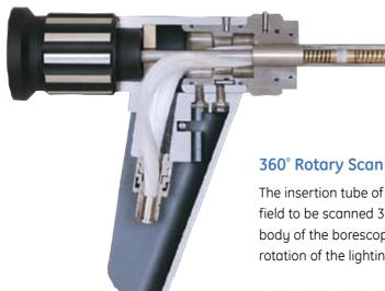
The insertion tube of the Rigid Borescope can be rotated, allowing the viewing field to be scanned 360° (with overlap from field-of-view) without moving the body of the borescope. A positive stop is built into the body to prevent overrotation of the lighting fibers.
