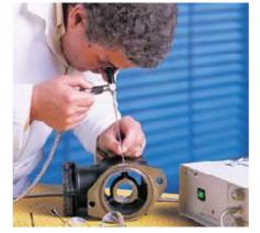
Inspecting air-brake compressor after machining
