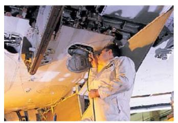
Inspection of hard-to-reach area of airframe structure
