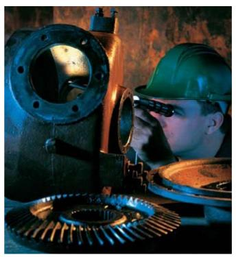
Rigid Borescope inspection of power take-off transmission
