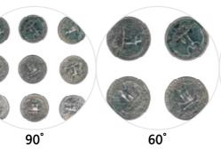
The 90° field-of-view, shown at the far left, produces the lowest magnification. The 60° and the 35° field-of-view provide increasingly greater magnification.
